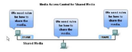
• Refers to controlling when computers can use the media i.e. when can they transmit and receive.
